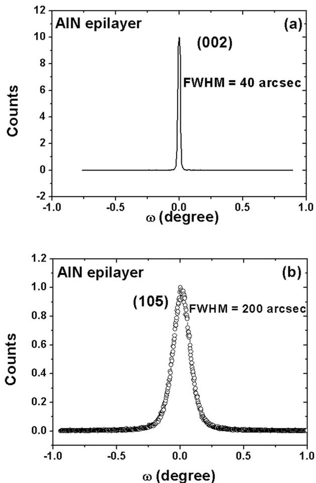
FIG. 4. X-ray diffraction  $\omega$  scan (rocking curves) of the (a) symmetric plane (002) and (b) asymmetric plane (105) of an AlN epilayer used in this study.
