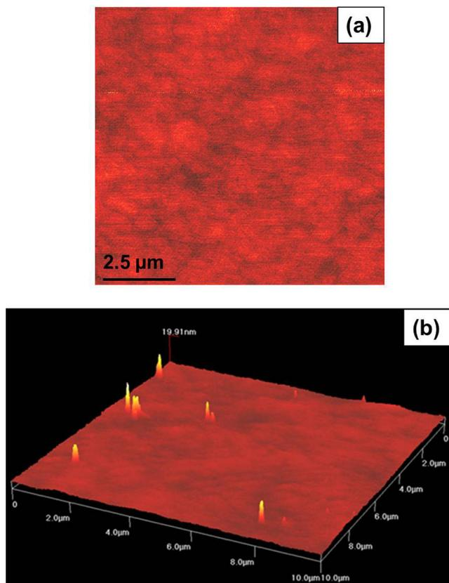
FIG. 2. (a)  $10\ \mu\text{m} \times 10\ \mu\text{m}$  AFM image of AlN epilayer grown on (001) SiC. Smooth surface with root-mean-square roughness 0.4 nm and (b)  $10\ \mu\text{m} \times 10\ \mu\text{m}$  AFM image of KOH-etched AlN epilayer used to evaluate the etch-pit density.
