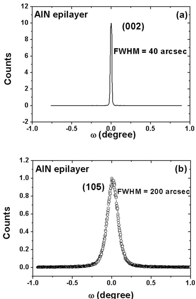
FIG. 4. X-ray diffraction  $\omega$  scan (rocking curves) of the (a) symmetric plane (002) and (b) asymmetric plane (105) of an AlN epilayer used in this study.
