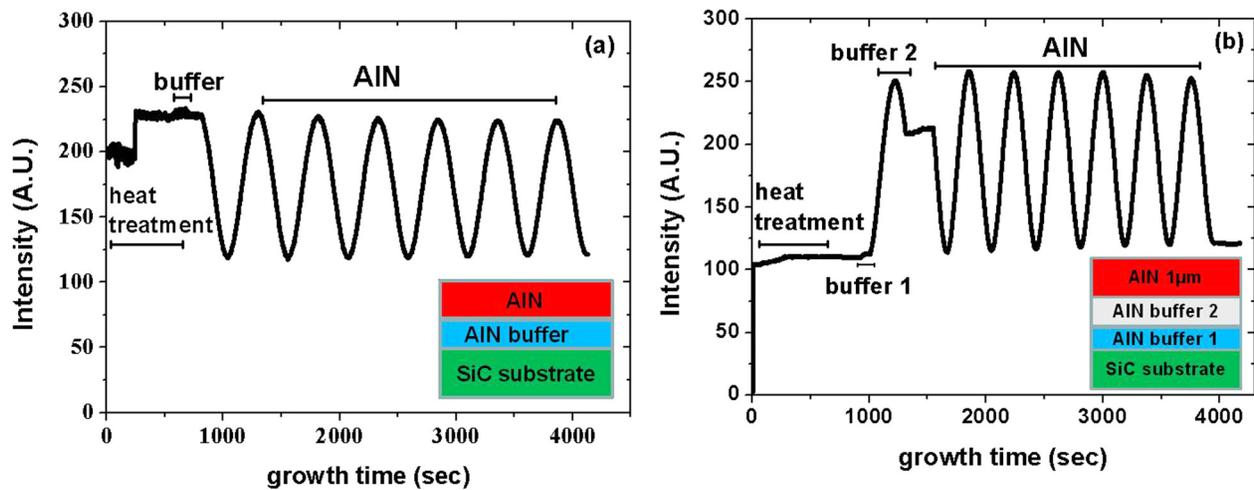
FIG. 1. *In situ* optical reflection curve during the growth of AlN epilayer by (a) single buffer AlN growth method and (b) double layer AlN buffers growth method. Inset: Schematic layer structure of single and double layer AlN buffers growth methods.
