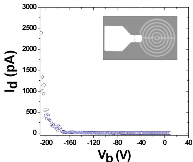
FIG. 5. I-V characteristic and the optical microscopy image of a fabricated photodetector with a device size of  $100 \mu\text{m}$  in diameter.
