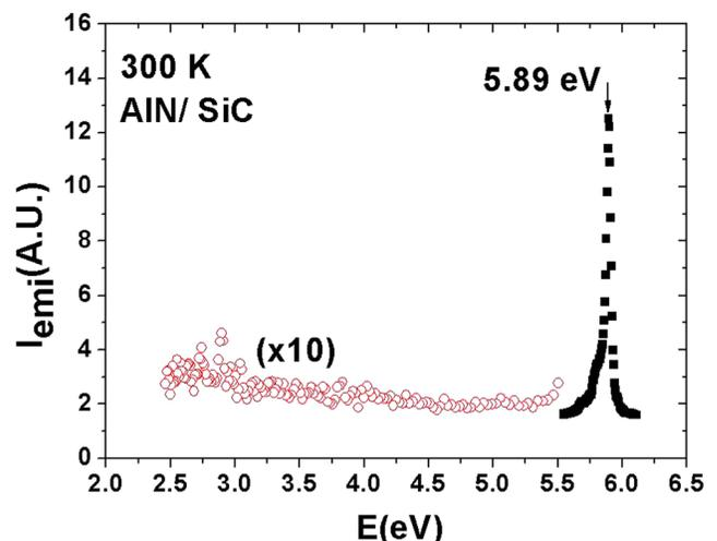
FIG. 3. Room temperature (300 K) photoluminescence spectrum of an AlN epilayer used in this study.
